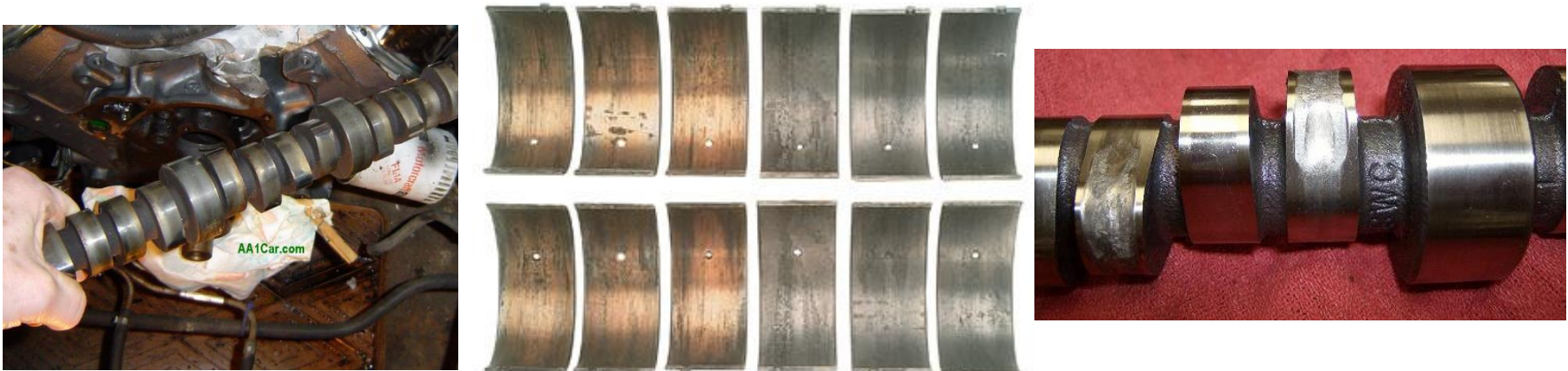
Oil starvation: very shiny surfaces and evidence of wiping
